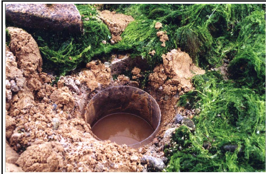
Figure 4. A temporary sampling well used to collect intertidal groundwater samples for virus and nutrient analysis. The plastic well casing is 8.25 inches in diameter and 14 inches in length. Samples were collected using a plastic submersible electric pump placed in the well. The green seaweed is probably a species of Enteromorpha .
